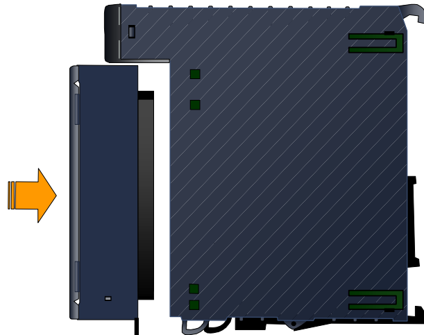
Figure 428: Installing a High-Density Terminal Block
