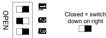
Figure 18: Example of Backplane DIP Switch Setting for Rack Number
