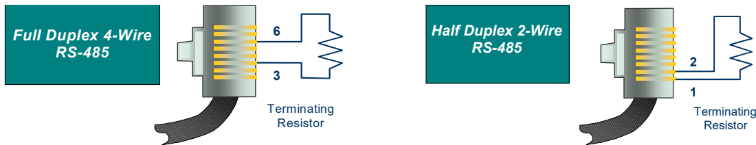
Figure 372: Termination RS-485 4-Wire Full Duplex
